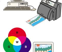
Television and Computer displays express various colors by combining three colors referred to as the three primary colors of light, namely red (R), green (G) and blue (B). Any color can be created with these three colors. In addition, mixing equal amounts of these three colors results in the color white (W).
